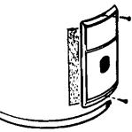
5. Open the flap of insulation to expose the opening.
